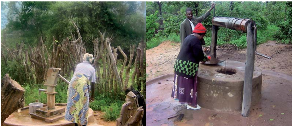
Figure 16: The two most common water point types: Handpump of type India Mark II (left) and hand dug well with bucket and windlass (right).
